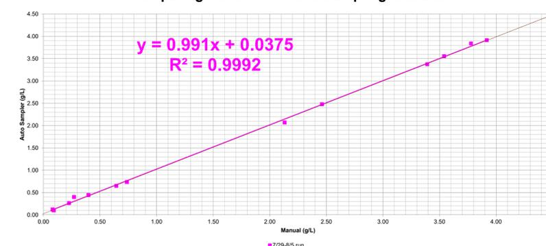
Figure 4. Comparing Manual and Auto Sampling When Lactate levels are monitored. The coefficient of determination is over 0.99, suggesting a strong correlation.
