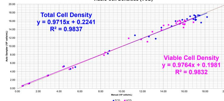
Figure 3. Comparing Manual and Auto Sampling focusing on Total Cell Density (TCD) and Viable Cell Density (VCD). The coefficient of determination is over 0.98, suggesting a strong correlation.
