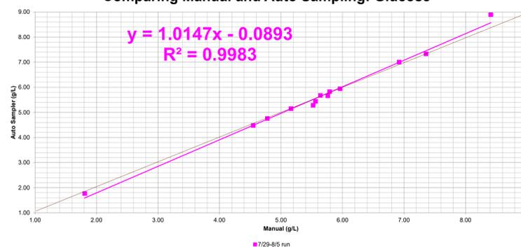
Figure 2. Comparing Manual and Auto Sampling When Glucose levels are monitored. The coefficient of determination is over 0.99, suggesting a strong correlation.
