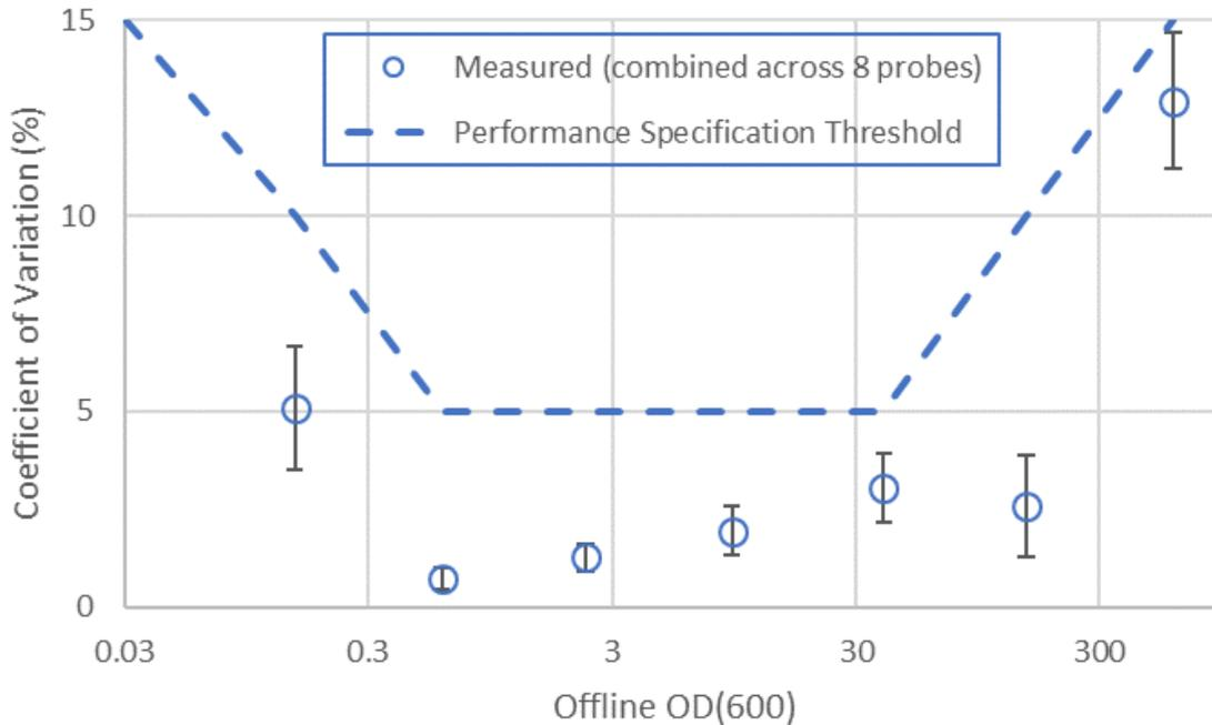
**The graph above shows the process-induced variation in yeast dry cell weight prediction across process conditions spanning the full range of a typical aerobic fermentation (200 mL vessel, agitation: 750-2000 rpm, sparge: 0-2 vvm).**
